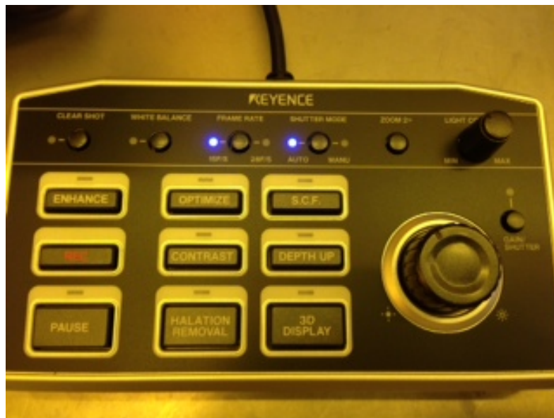
11.2 Control console is pictured. Definitions of the buttons are found in section 4.
