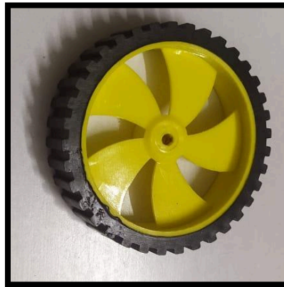
Fig. 7.4: Nylon Reinforced Rubber Wheel
