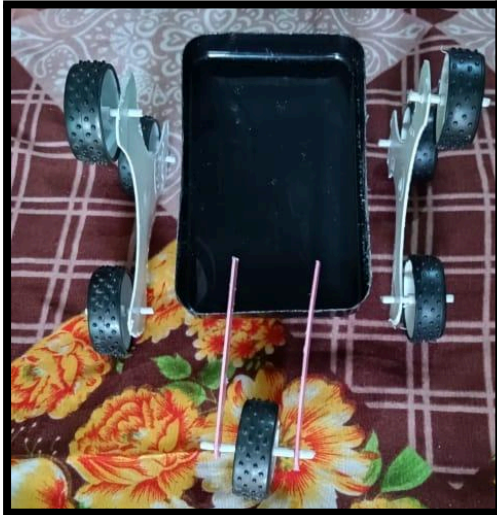
Fig. 7.14: Initial Design of MTCV with PP Frame
