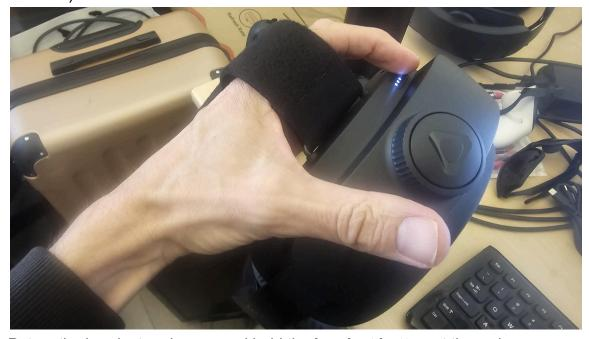
Put on the headset and press and hold the headset button at the welcome screen. • Pair controllers as prompted.
