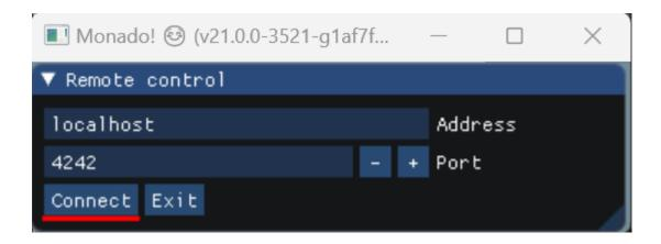
An interesting feature of the Remote Control window is you can use an IP based network computer connection to drive the OpenXR session externally.
