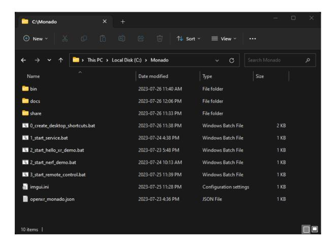
I created several .bat scripts to streamline the process of launching the OpenXR Monado service, the remote control GUI, and a sample Khronos group produced OpenXR program called "Hello XR" that displays several colourful cubes in a stereoscopic 3D environment.
