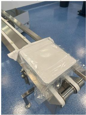
The tub has to be adjusted inside the bag and the flaps of the bag need to be spread out. It is common to have the tub not adjusted correctly and then placed onto the line where it has the potential to stop the line due to its placement. Reducing the amount of downtime from this issue would greatly help line efficiency while reducing potential operator strain.
