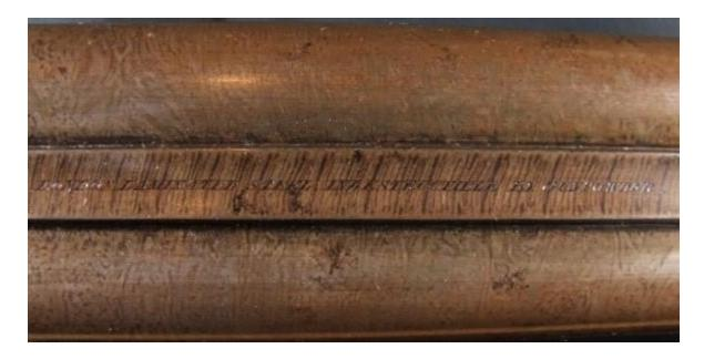
c. 1880 W.W. Greener "The Trap Gun" with (non-Silver) Laminated Steel courtesy of Leighton Stallones. Note transition to the mid-barrel tube segment.
