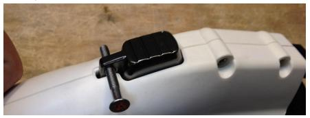
2. **Be creative but careful in this part** - you should now apply upward force on the latch end to bend it straight. The metal may break if a striking force is used (e.g. a hammer), or if bent too far. Be careful not to bend it too far, though you can correct it by pushing both ends down instead of up.
