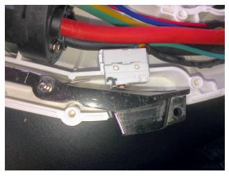
4. Seal it back up by placing the upper housing back onto it, making sure to re-attach the rubber plug protector if desired. Note that two of the Torx screws are smaller than the others - those go in the two holes at the bottom, closest to the cable.
