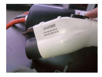
3. Take the J1772 plug apart, making note of the two smaller screws by the cable inlet:
