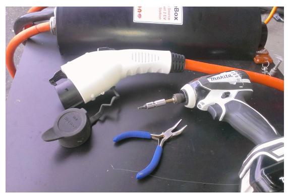
2. You can test lever action to see that switch clicks about half-way through the locking hole. If it clicks quicker upon pressing the button (before half-way through the lock hole), there's a problem to fix.
