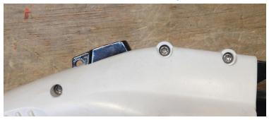
This damage is evident by the lock-hole not being fully visible when the lever is released, but the lever still presses and releases smoothly (though not a full range of motion).
