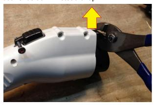
When the lever is properly straightened, the latch end should travel the full range of motion within the plastic handle body cut-out, and the proximity switch should "click" around half-way through the lock hole travel. The lock hole should be fully exposed when released.
