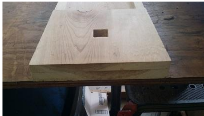
Figure 12 The square mortise for the anchor.
