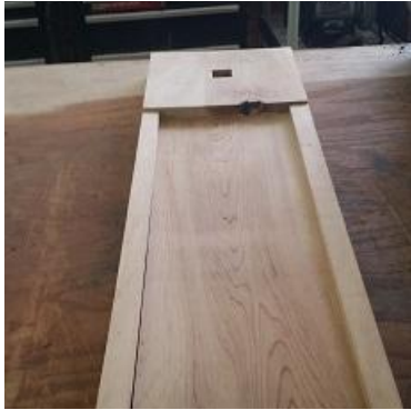
Figure 13 The base after assembly of the riser and rails.
