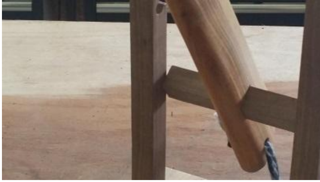
Figure 10 The beater placed where their supposed to be. This is from my first foot beater and the uprights are swelled into place so I can't remove them to put the beater in the correct place.
