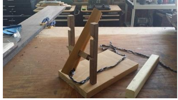
Figure 4 Where the rotation point is supposed to be for the beater. The cutouts are for a stopper to send the beater back down. The biggest omission from almost all drawings.
