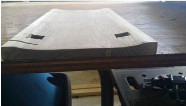
Figure 5 On the left my first sled. Notice the concave shape of the bottom. This design was very detrimental in making a working foot beater.
