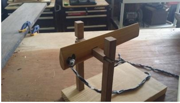
Figure 3 Where I initially put the rotation point for the beater.
