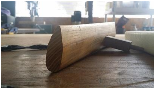
Figure 9 The beater shape with the rotating rod in place.
