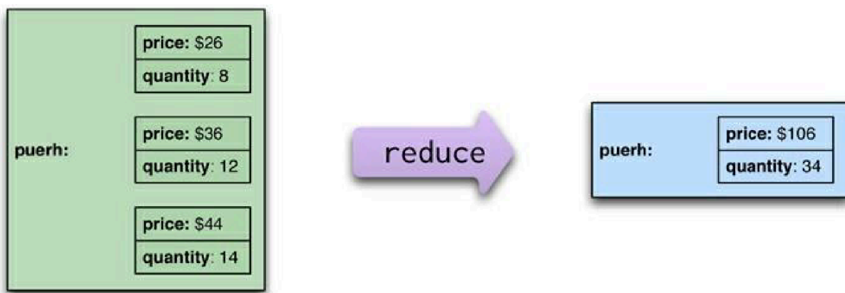
Figure 1.2. A reduce function takes several key-value pairs with the same key and aggregates them into one.
