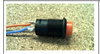
Cut 2 40mm wires using different colors if available.
