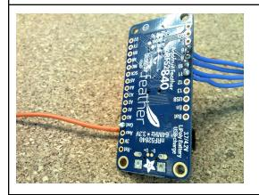
**Cut** a 40mm long wire and **solder** it to the Ground pin on the feather board.
