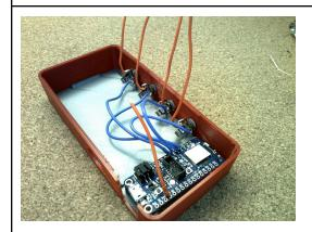
**Insert** the mono jacks into the case and fasten them into place using the provided rings.
