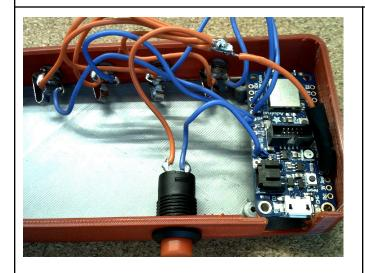
**Insert** the button into the available hole in the case and fasten it into place using the provided ring.
