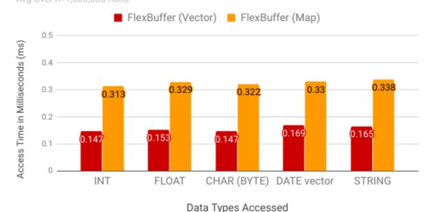
The results show that vector-based FlexBuffer has a considerably faster access time for each tested data type over the map-based FlexBuffer (52% on average). However, the use of vectors would require some mechanism for tracking whether any fields are missing/null within the FlexBuffer. We can track null
