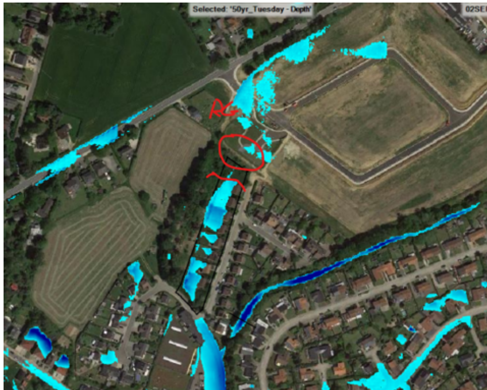
Figure 21: applying Culvert strategy for area id code- 427.
