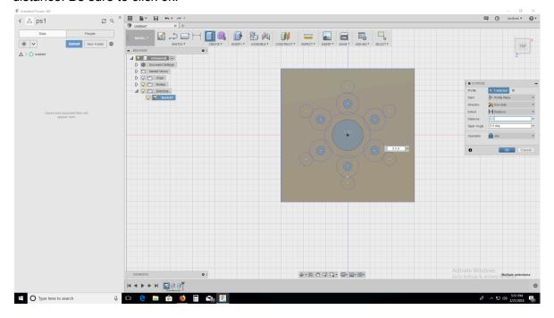
18. Click the 'orbit' button in the center on the bottom, select the base and orbit the object to view the design. You can also orbit by clicking and dragging the cube in the upper right.
