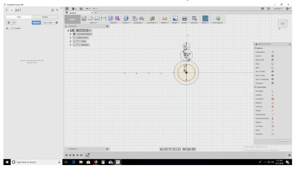
10. Under sketch, select 'circular pattern', a menu will appear on the right. Click the outer ring on the 1" circle and the ring on the circle within the 1" circle. In the 'circular pattern' box after 'objects it should indicate '2 selected'. Click in 'center point' and click on the dot in the 2" circle. Three circles should appear, change the quantity to 6. Click OK to save.
