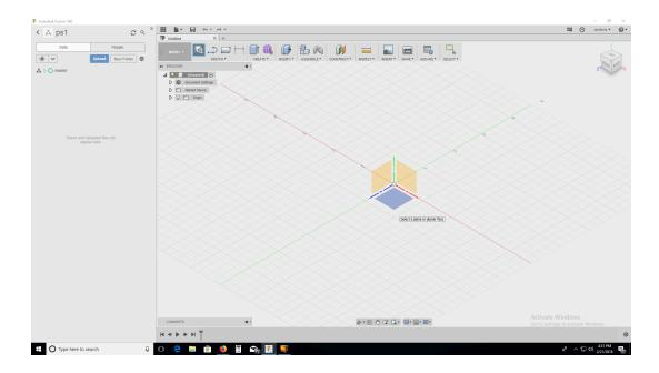
4. The view will change to plane selected, in this case 'top', notice in upper right it indicates 'top'. Buttons in the bottom of the screen control the view. If needed change the grid to inches, 1 in per major line.
