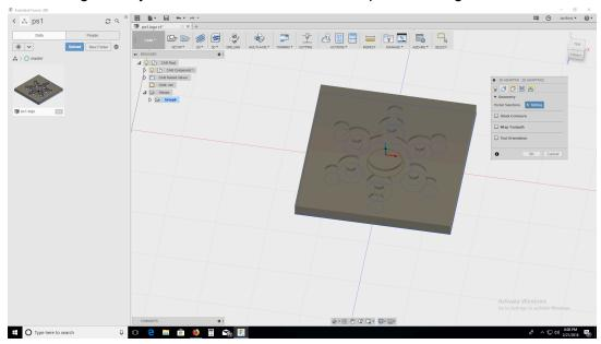
27. Move the arrow over the design until the design lights. Click to choose the chain for pocket selection. If any part of the design did not light move the arrow to that part and click to select.
