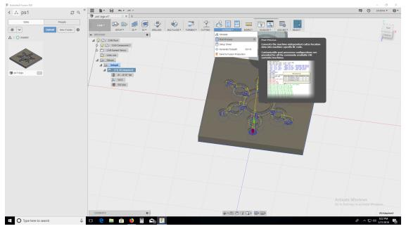
32. I used the Easel post processor saved on my machine. Other processors may work but I have not found a loaded processor that works.
