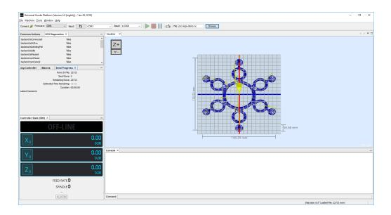
35. Select the correct port and press the connect, it should change to 'disconnect' and several messages will be displayed in the console.
