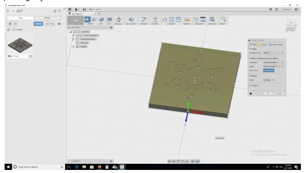
22. Click on 'model orientation' in 'Orientation' of the dialogue box. Select 'z axis/ plane and y axis' option. Click it, then move the arrow to the body of the object and click. The z axis (blue) should change to up. The y axis (green) points to the back and the x axis (red) across. Click ok to save this orientation. This matches the orientation on a mill, the z axis is the spindle, the x axis the table side to side and the y axis table front to back.
