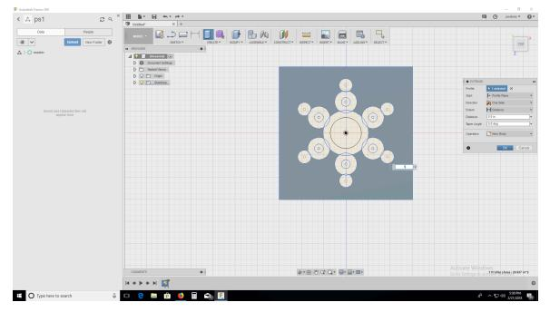
16. Click on 'sketches' and make sure 'sketch 1' on in the drop downs on the left . Then select 'create' and 'extrude' and select each of the circles indicated in the following screen print. Enter a distance of .375 and click OK.
