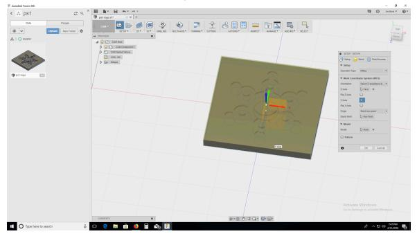
For more help orienting the Z axis to point upward, mouse over "Orientation" for the following direction pop-up. Click the 1st "Select Z axis/plane" option of the two.
