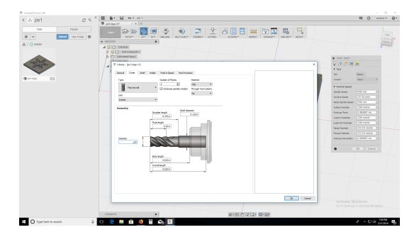
26 Select 'geometry', the second button in the 'adaptive clearing' box.
