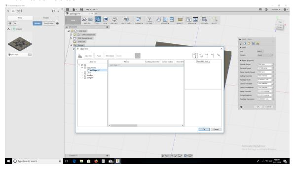
25 For a ½ sq end mill select the 'new mill tool' at the top. You will get a screen to define the mill. I selected type 'sq end mill', changed the unit to in, number of fluites to 2 and changed the diameter to .125. Click ok to save the tool definition.
