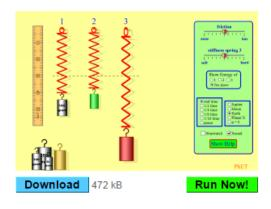
12a. Grab a spring, a force sensor, and be careful not to overstretch the spring (seriously). What is the relationship between the Force applied to a spring and the amount it stretches? What variables will you need to measure? (Use a Labquest 2 or the Lab Pro)
