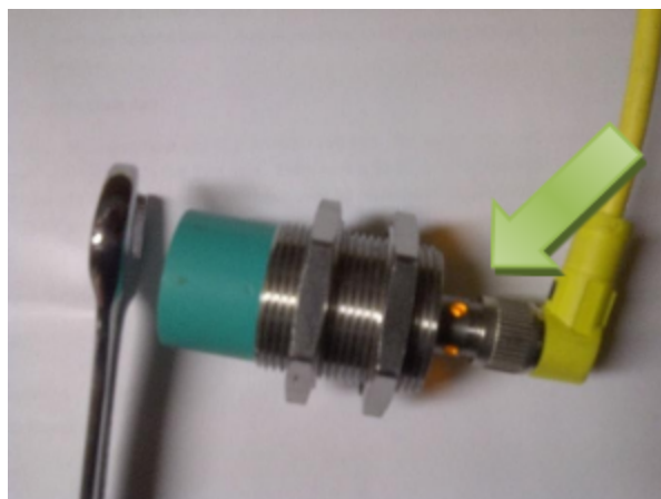
Proximity sensor – when powered, will detect metallic objects within ~1/2" from the sensor, depending on make and model.
