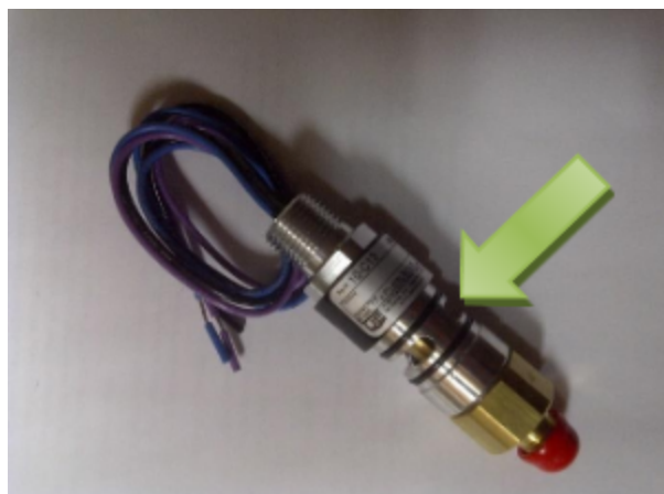
Hydraulic sensor – sensitivity range of 100-1500 PSI, which can be adjusted by twisting the central shaft (see arrow).
