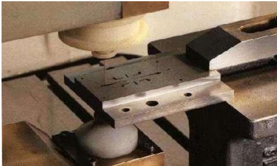
Figure 4: Wire erosion of an extrusion die
