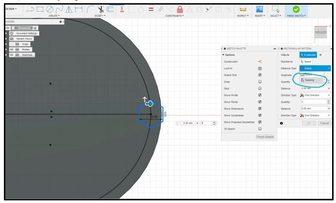
9) Pattern one hexagon horizontally, this is so you have an object to reference a direction later on
