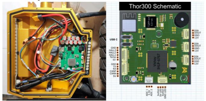
I chose the CNC box because machined aluminum has double the thermal conductivity of die-cast aluminum (~180 w/m.k. vs. ~90 w/m.k.), which means my controller will be less likely to overheat.
