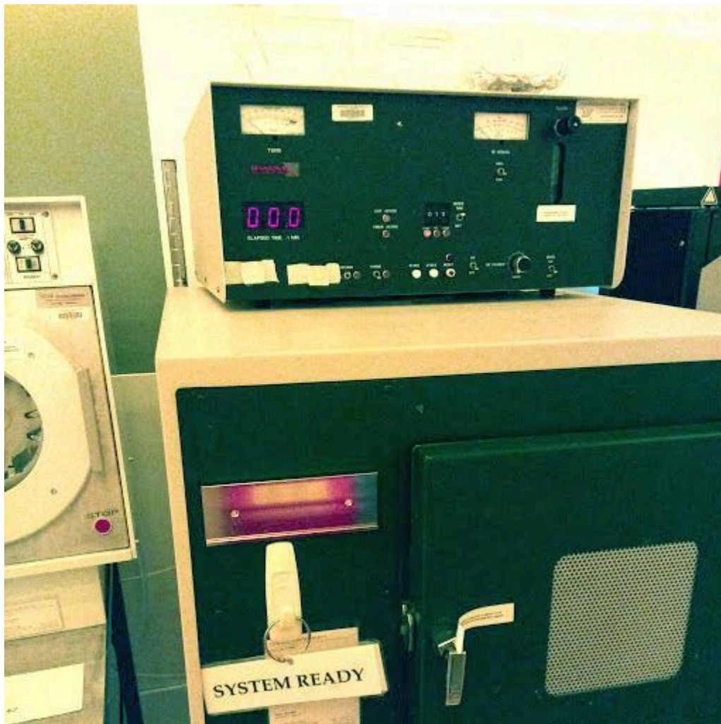
Figure 1 The oxygen asher, located in Keller Hall-Bay 2.
