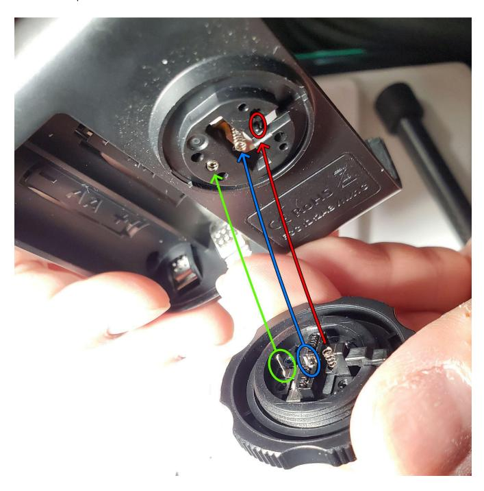
22. Place a finger on the metal hotshoe so it doesn't fall out. Then reinstall the 4 screws circled green. Ignore the red circles here.
