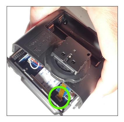
5. At the power button side, there's a power connection. Gently pull it up and out. I simply pinched my fingers on the wires and pulled out the connection.
