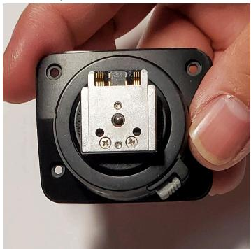
2. Remove 4 screws covered in this white stuff. I didn't bother to remove the white stuff. I just jammed my screw driver bit into it and unscrewed them.
