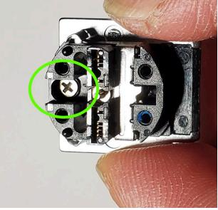
14. Insert the metal hotshoe into the plastic piece so that the notches align.
