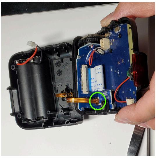
22. Install the power connector. The connector is directional so you can't install it incorrectly.
