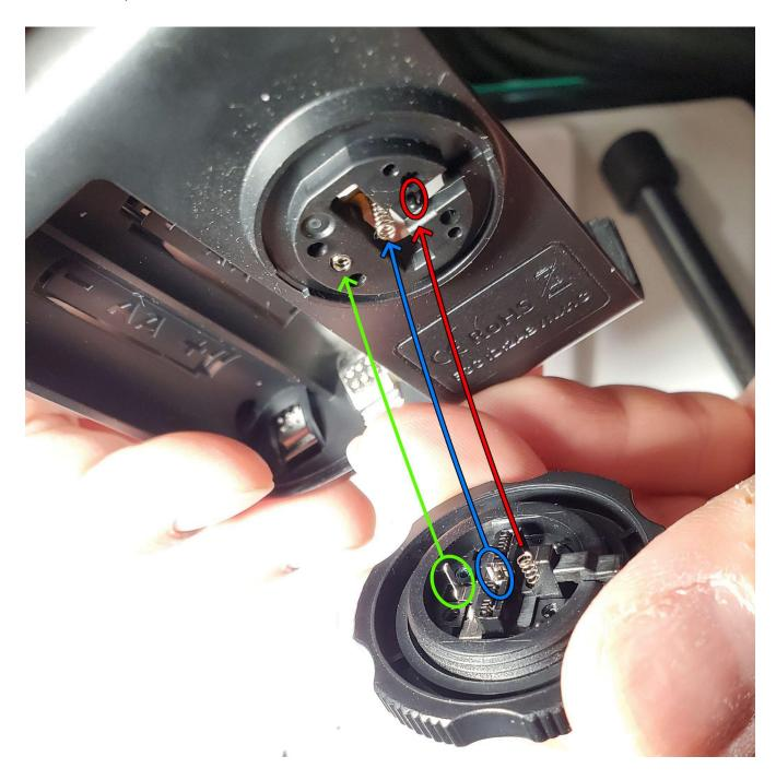
20. Place a finger on the metal hotshoe so it doesn't fall out. Then screw on the 4 screws circled in green. Ignore the red circles.
