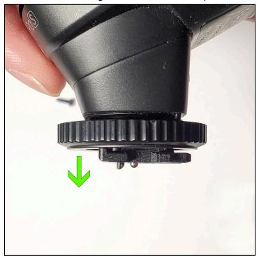
3. Pop open the trigger from the front. Becareful not to dislodge the power buttons here.
