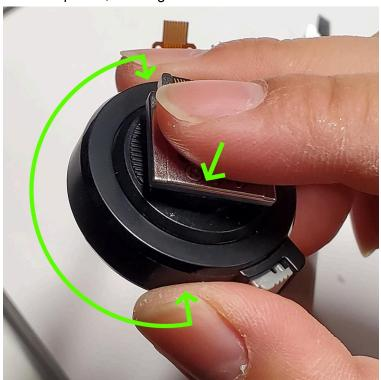
6. Once the 4th screw circled in green is removed, tilt the shoe so it's sideways like this.
