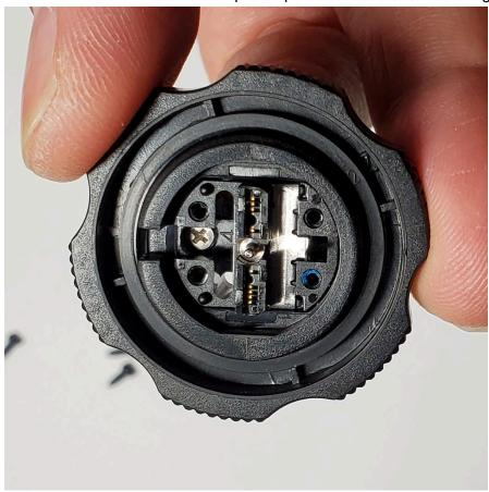
18. There is a hole circled in green, put the plastic fork piece into there. It may be snug, so push it down so it's as flushed as can be.
