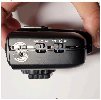
4. At the rear of the device, the hotshoe ribbon is connected here. Use your fingers to hold the ribbon and pull it up and out. If your fingers can't access the ribbon, you can wrap cloth / tissue around the points of a tweezer to pull the ribbon up and out.
