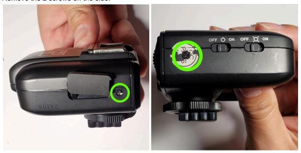
3. SLOWLY Pull apart the plastic covers. Becareful so that the power buttons don't break off. Becareful not to yank on the ribbons and wire inside.
