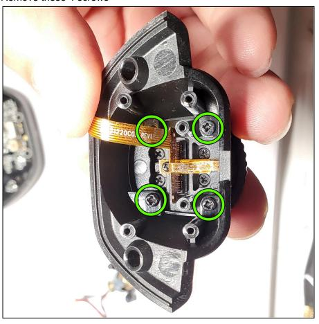
8. Put a finger under the plastic hotshoe before removing all the screws in the next step
