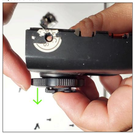
7. Before removing the plastic hot shoe, I would support the plastic hot shoe with a finger so it doesn't drop out.
