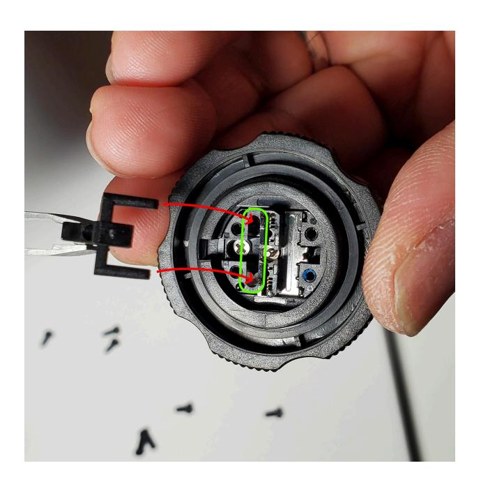
19. Remember the removable spring in step 12? Take it and insert it into the hole of the plastic fork piece.
