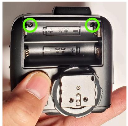
2. Remove the 2 screws on the side.
