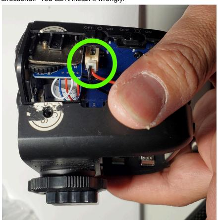
6. Let's work on the plastic cover that contains the hot shoe. Rotate the locking wheel so that it lightly stops at the hotshoe.
