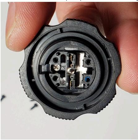
16. There is a hole circled in green, put the plastic fork piece into there. It may be snug, so push it down so it's as flushed as can be.
