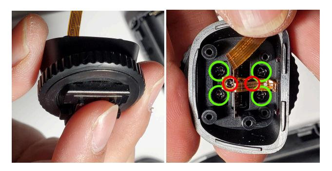
21. Install the ribbon that goes into the metal hotshoe. I alternated between these two green points to push the ribbon into place. Do so gently so you don't damage the ribbon.
