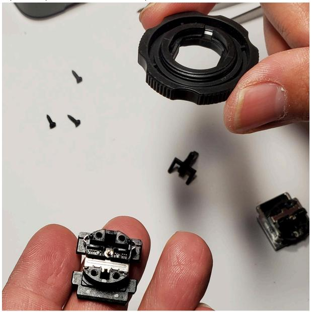
13. Take the metal hotshoe and prepare to install it into the trigger assembly. If the center pin fell out, this is the orientation to put it back in.
