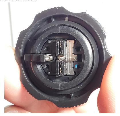
19. Now we'll take this metal hotshoe assembly and combine it with the lower piece of the flash trigger. Notice the GREEN line. There's a metal prong that must go INTO the spring here. Notice the BLUE line. The center pin must go INTO the spring here. Notice the RED line. The spring must go into the black plastic pin here.
