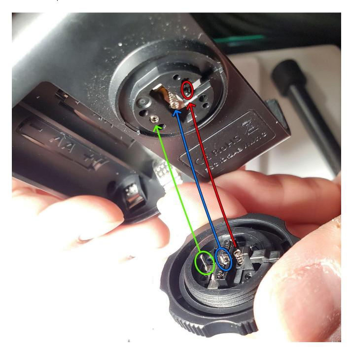
19. Place a finger on the metal hotshoe so it doesn't fall out. Then screw on the 4 screws. To hold the hotshoe assembly.
