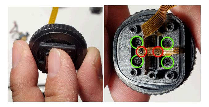
23. Picture from a different install. Install the ribbon that goes into the metal hotshoe. I alternated between these two green points to push the ribbon into place. Do so gently so you don't damage the ribbon.
