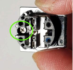
17. Insert the metal hotshoe into the plastic piece so that the notches align.
