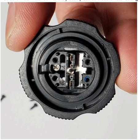
15. There is a hole circled in green, put the plastic fork piece into there. It may be snug, so push it down so it's as flushed as can be.
