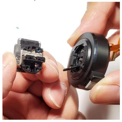
8. There's a metal pin at the center of the metal hotshoe. In case it fell out, here's the correct orientation to put it back in.
