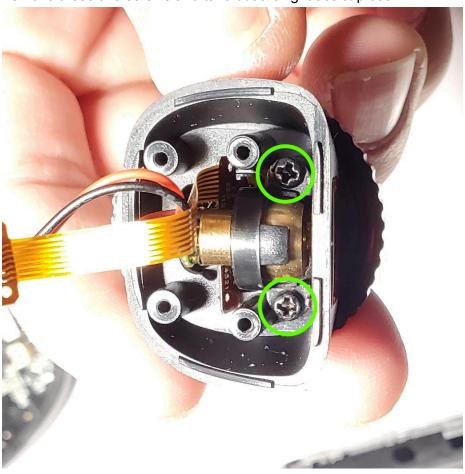
7. Put in a finger on the plastic hotshoe like this, so in the next step, the plastic hotshoe doesn't fall out uncontrollably.
