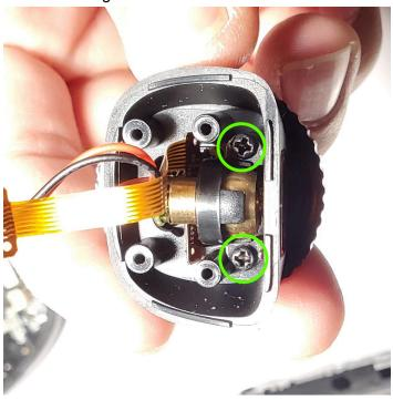
23. Reinstall this assembly into the lower cover of the trigger
