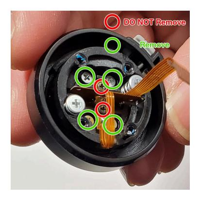
5. How to hold the piece before removing the last screw circled in green above. Two fingers on the circle plastic, one finger on the metal hotshoe.
