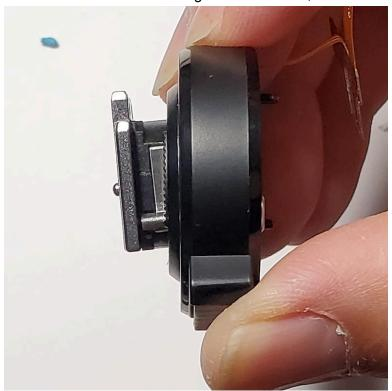
7. Slowly pull apart the metal hotshoe from the plastic housing. Wiggle gently if you have to. The most resistance you'll face is the ribbon that's connected to the metal shoe.
