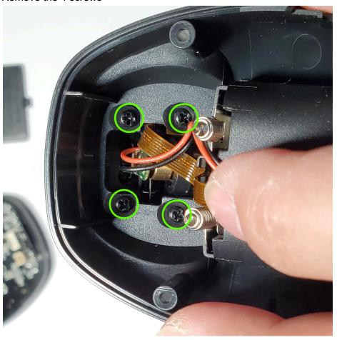
6. Remove these two screws and take out the light assist piece.
