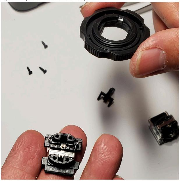
12. Take the metal hotshoe and prepare to install it into the trigger assembly. If the center pin fell out, this is the orientation to put it back in.
