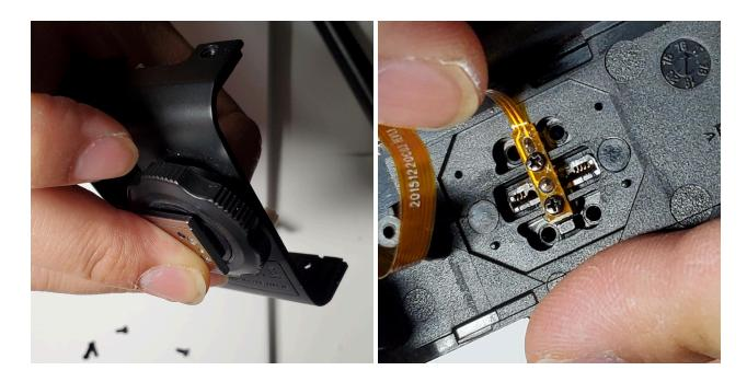
20. Install the ribbon that goes into the metal hotshoe. I alternated between these two green points to push the ribbon into place. Do so gently so you don't damage the ribbon.
