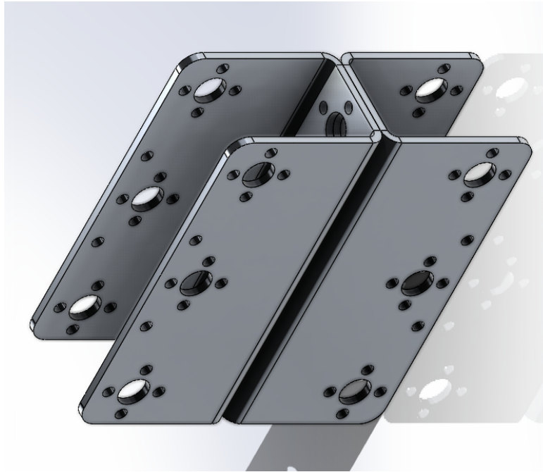
Figure 19: Brackets to Attach Servo Motors to Case
