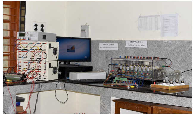
dSPACE 1103 Real Time Digital Controller
