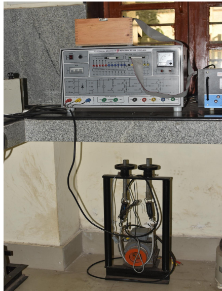
Electrical Braking of 3 Phase Induction Motor (VPET-405)
