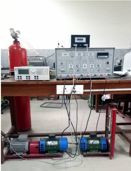
Ward Leonard Speed Control System Transfer Function Study Trainer (PEC14HV2)
