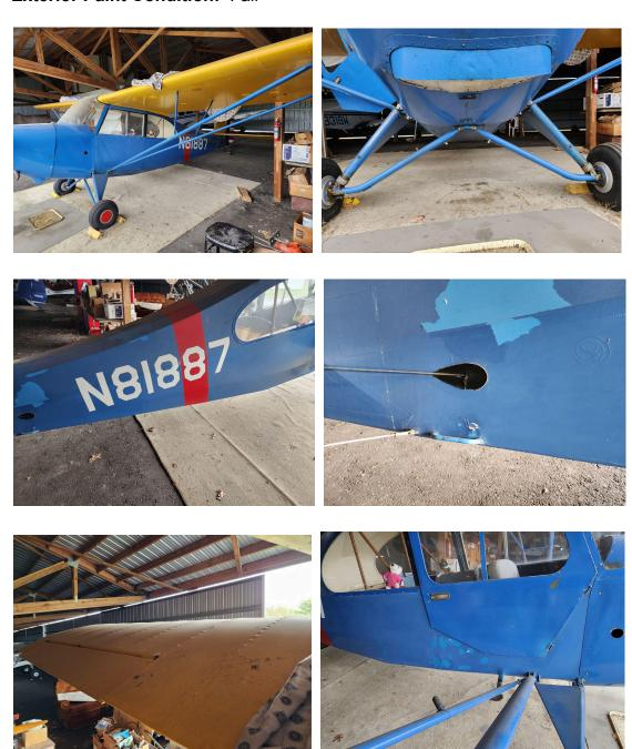
**Comments:** In June of 1983, the fuselage and horizontal & vertical stabilizers were recovered. In June of 1994, the fabric control surfaces were refinished. The tires are in very good condition, they still had the little nubs on them.
