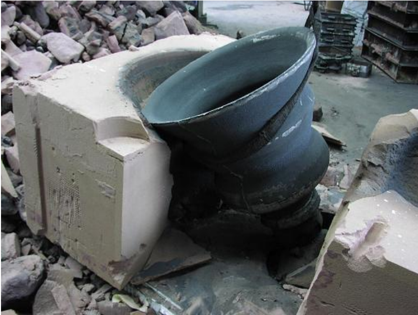
Figure 14 One half of a Time and Tide Bell being broken out of the mould
