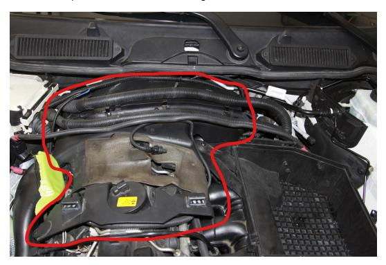
8. Disconnect the vacuum line (pinch connector)
