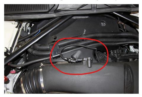
b. Pull back on intake clips (only for stock intake)
