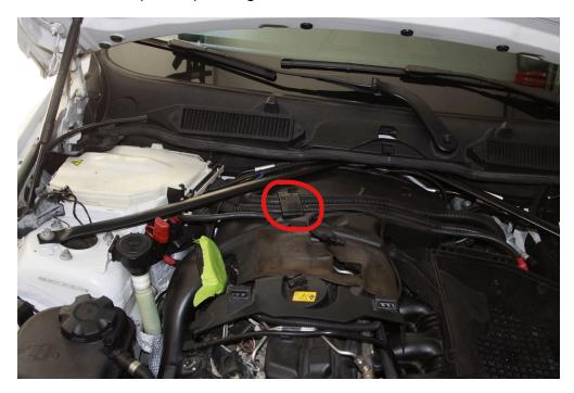
b. Pull up on the rubber grommets holding the 3 wiring looms
