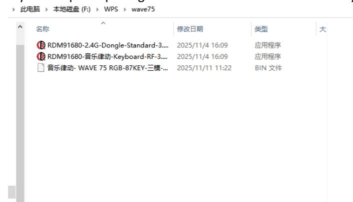
2. Flip the power switch to OFF, then press and hold the ESC key while powering on. A USB drive will appear on the keyboard's onboard storage. Once this USB drive appears, you can upgrade your keyboard.
