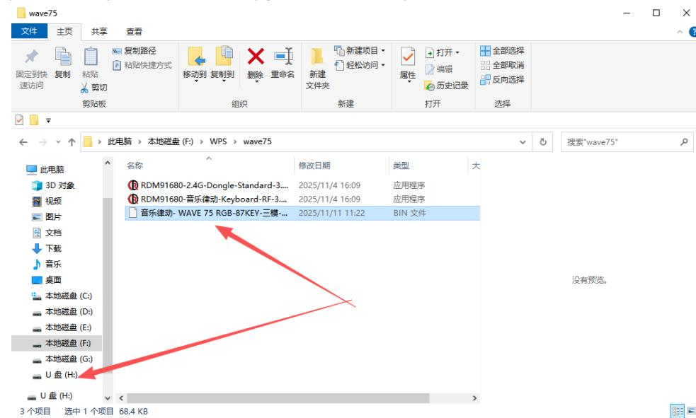
5: 2.4G Wireless Receiver Upgrade: Plug the receiver into the computer's USB port, open the receiver upgrade software, and click the Device info button. After clicking, it will display OK. Then, click the middle button to start upgrading the 2.4G receiver. When the progress bar reaches 100%, the upgrade is complete. Turn on the keyboard power switch, place the receiver on the keyboard, and press and hold FN+4 (until the 4 key light flashes rapidly). Plug in the receiver to pair successfully.
