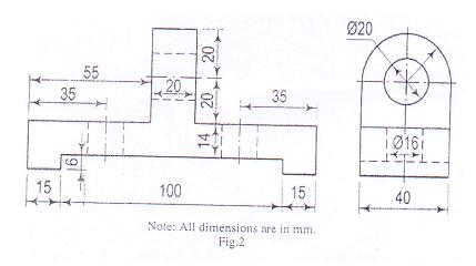
5. Draw the (i) Front view (ii) Top view and (iii) Side view for the following figure.
