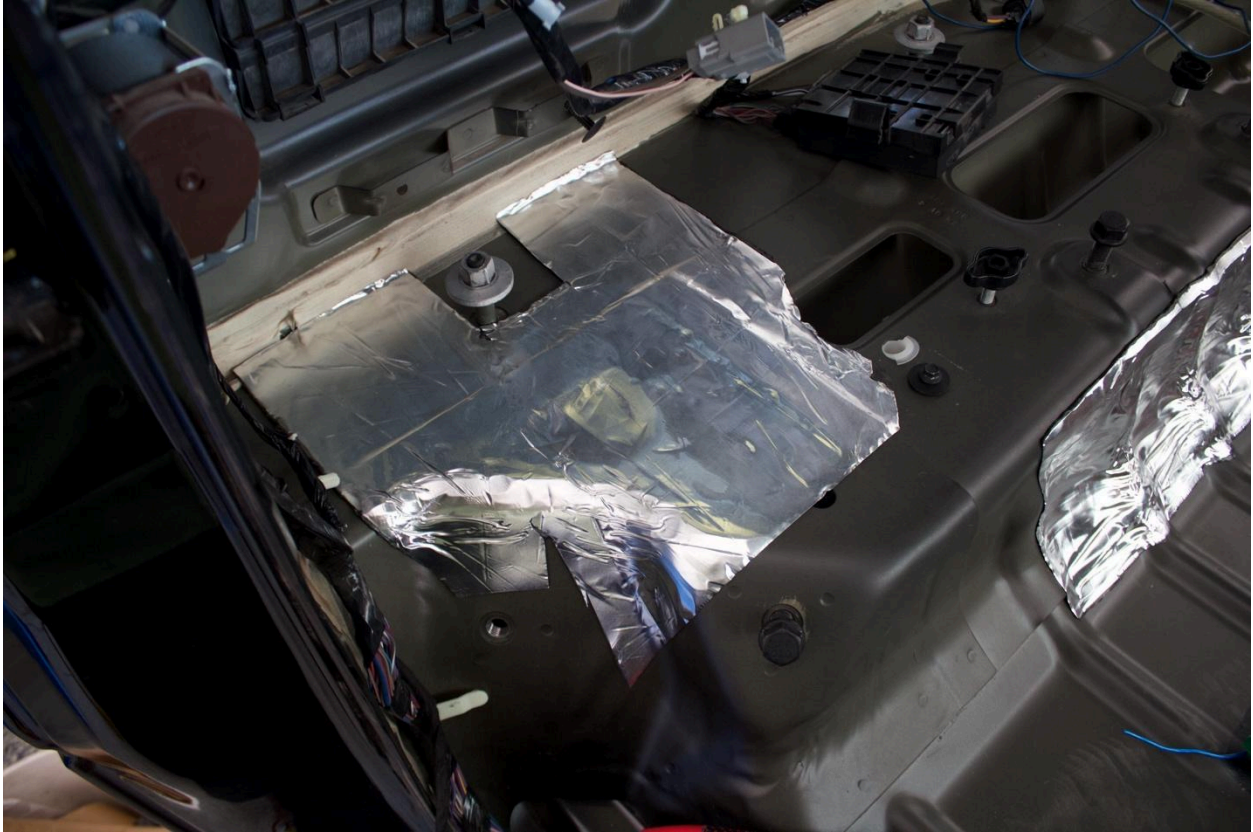
The seat platform also received 3 CLD squares
