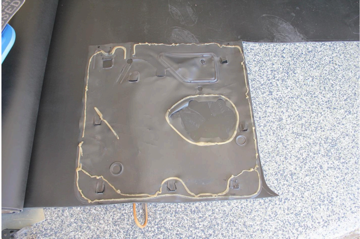
Trace the vapor barrier on the MLV and CCF
