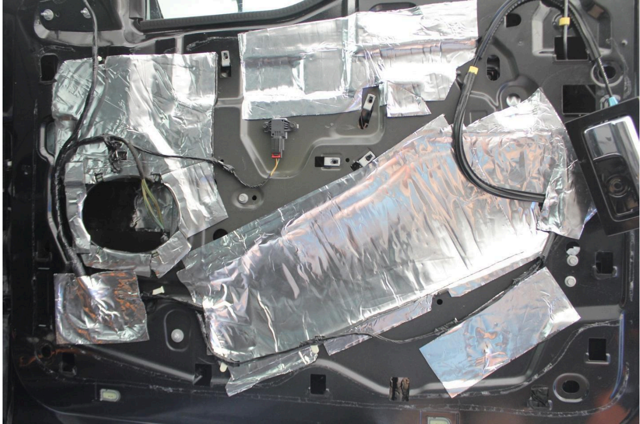
I then used 1 CLD square on the outer skin and 1.25 CLD rectangles
