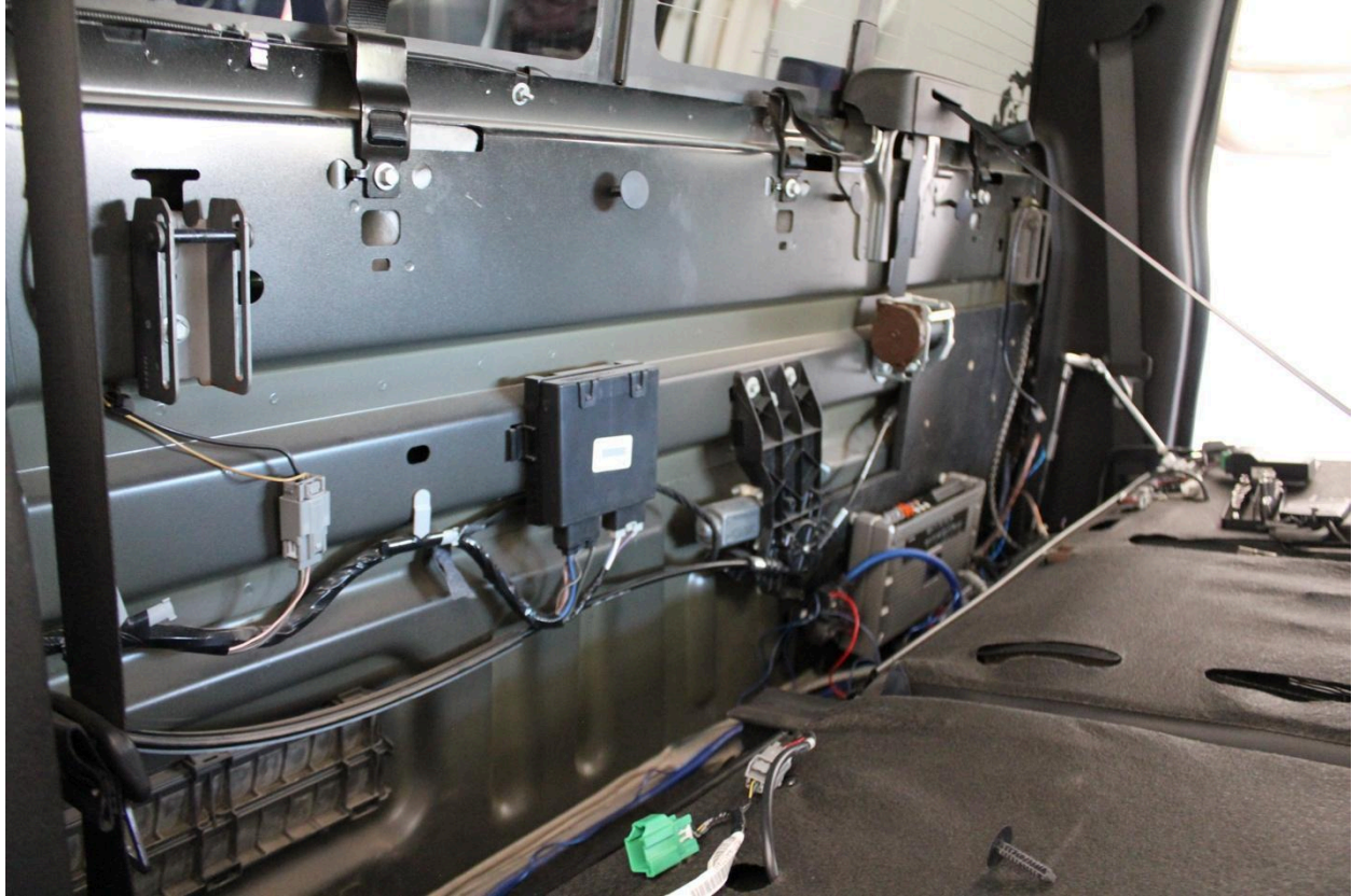
Remove back wall carpet so you can access the rear seat bolts. This is just pine tree clipped in place.
