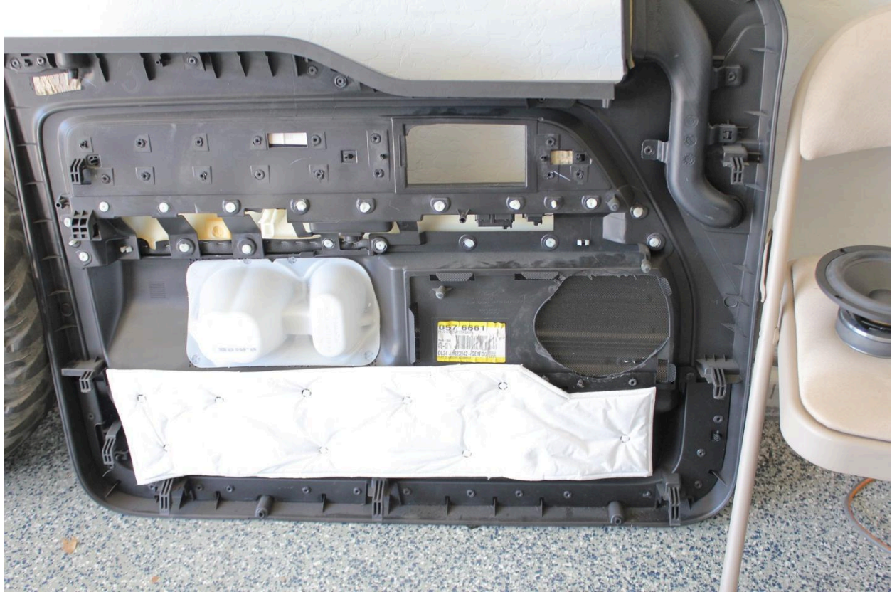
The door card had 1 CLD Square and probably about .25 rectangles. The factory fiber mat has some weird clips so it wasn't removed. But you can lift it carefully and place some CLD under it.
