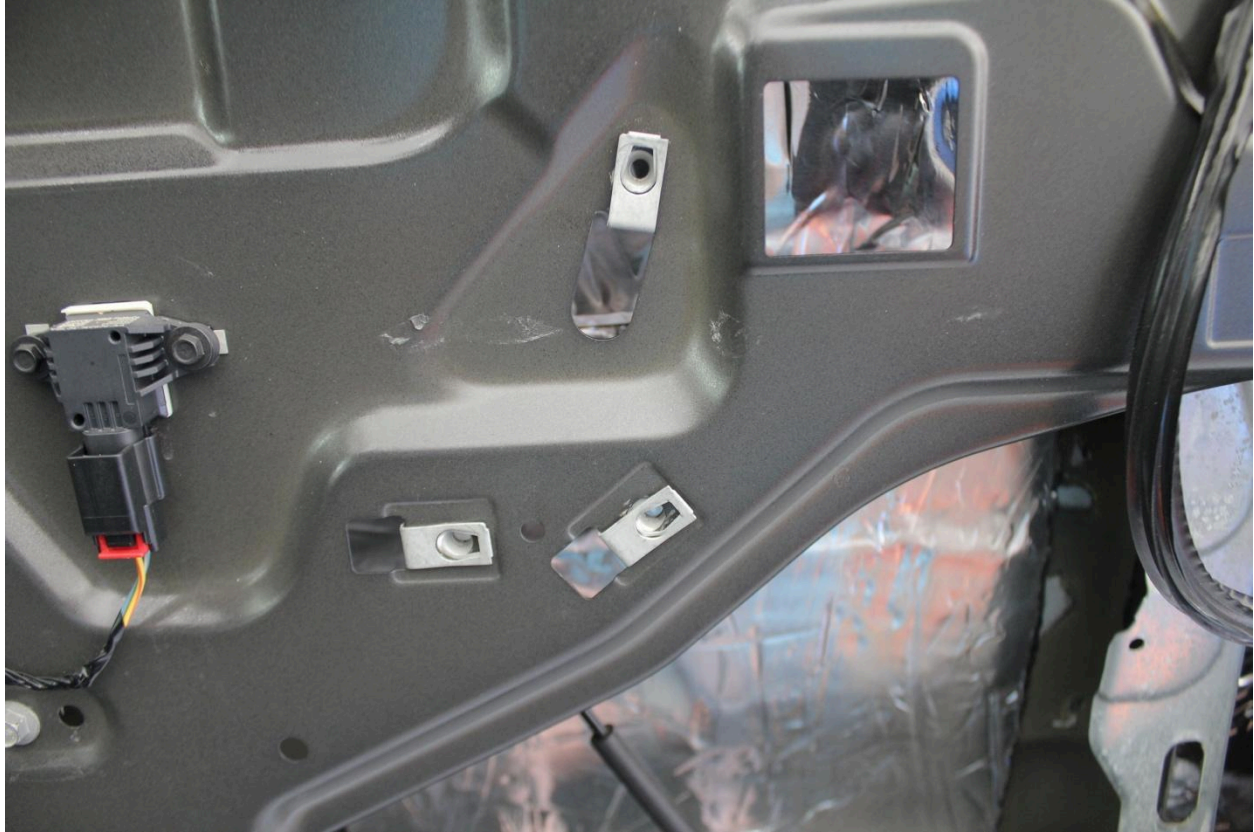
The outer skin now has some of these clips that like to wiggle and move so they got TESA tape to stop the noise.
