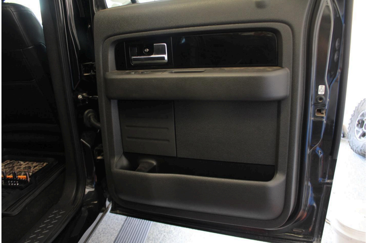
Similar with the rear door. Two 6mm bolts on the bottom, 1 8mm bolt in the door handle. No bolt under the grab handle but there is one at the top right.
