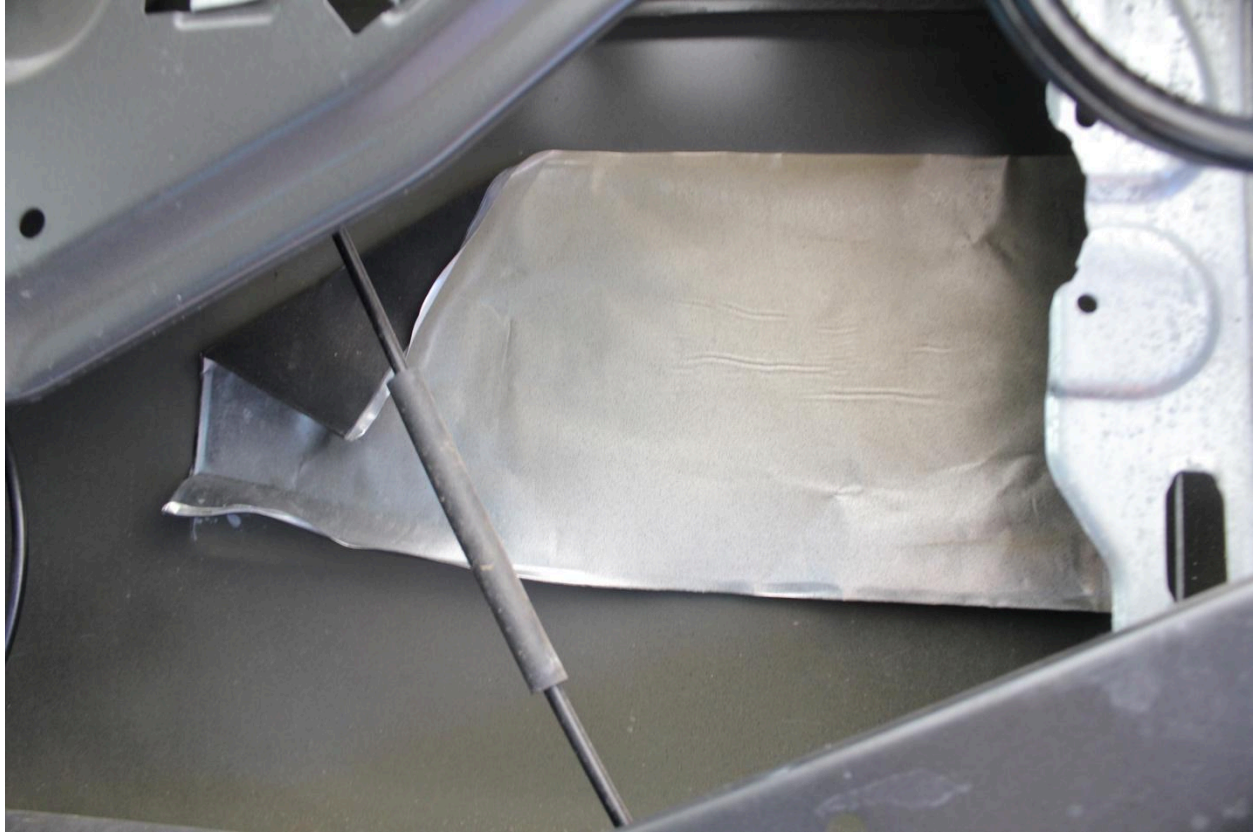
The factory CLD was falling off the two front doors so it was removed.
