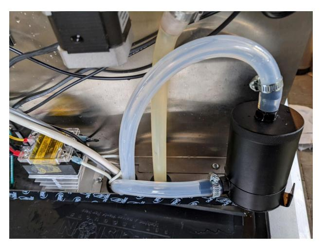
On the other side of the hole will be the final place for the reservoir. Thread the clamps over the tubing and connect the tubing as shown - the "L" shaped tube to the bottom port and the longer tube to the top - just to get the position right. You can screw down the lower clamp, but leave the top tube unclamped - this will be where you add the new glycol.
