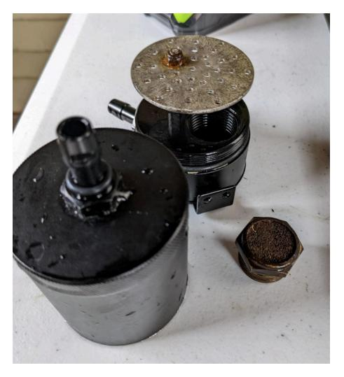
There is a brass filter inside the reservoir. This is not necessary for using this purpose, and if you leave it in, it will create resistance in the line, the glycol will not circulate properly and will give an error. The reservoir itself can be unscrewed by hand (just turn the top part counterclockwise from the bottom), but you will need an adjustable wrench to remove the filter.
