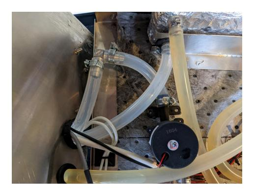
Connect the tubing on the inside with clamps as shown - the drain tube (L shape) connects directly to the glycol pump, while the longer run is connected to the heat exchanger. Note that it can be tricky to connect the tubing to the pump as it is seated. It can be helpful to remove the four screws securing the pump to the base, so that you can lift it up and seat the tubing appropriately.
