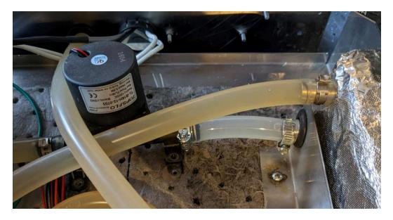
You will need to thread the new tubing through the place where the wiring is routed. It may be a tight fit, but there should be enough space to route the new tubing.
