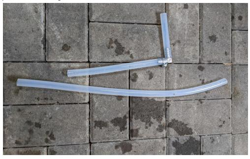
Looking inside the Zymatic, you'll see a short piece of hose connecting the pump for the glycol to the HEX (heat exchanger). This will likely have two Oticker-style clamps that need to be cut off to remove the tubing. Before you do this, elevate the left side of the base, so that this tubing is above the rest of the heat exchanger. This is not 100% critical, but will keep you from losing more glycol than necessary when you do remove the tubing.
