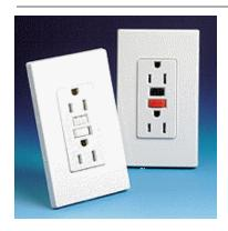
If current leaks through a person's body, it could cause ventricular fibrillation and electrocution. A GFCI stops current flow in a circuit when it detects leakage current to ground.
