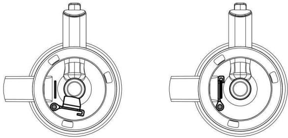
1, assemble bowl onto the base. Put bowl on the base and clockwise rotate to lock the bowl. Make sure the bowl is always locked on the base tightly. See below fig.
