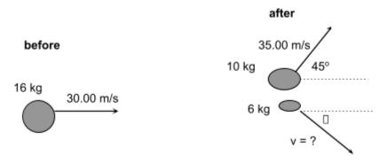
a. Calculate the total momentum before the explosion in each direction.
