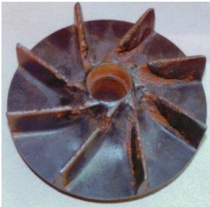
Fig.1.20.of damage was caused by imploding air bubbles.
