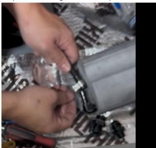
II. Connect lift pump connector
