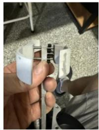
Put a m3x25 SHCS into the middle hole. You can remove the spacer once the middle is threaded through completely and the spacer is snug enough to slide out.
