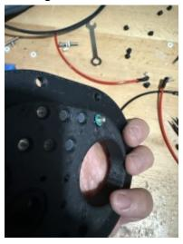
IV. Stack a washer on top of that o-ring
