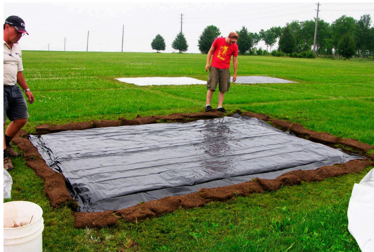
Figure 2 The polyethylene was put in place and the sod strips were placed over the edges of the poly and anchored in place using sod staples. (Charbonneau, 2011)
