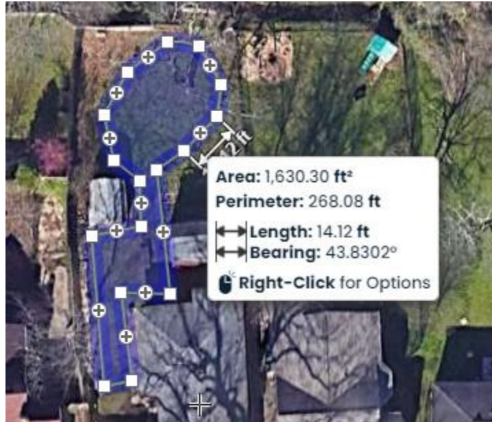
Figure 15 shows the pop-up box displaying the lawn measurement
