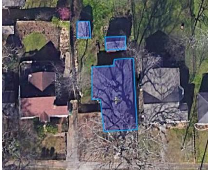
Figure 7 shows multiple closed polygon shapes (in blue) for buildings and sheds
