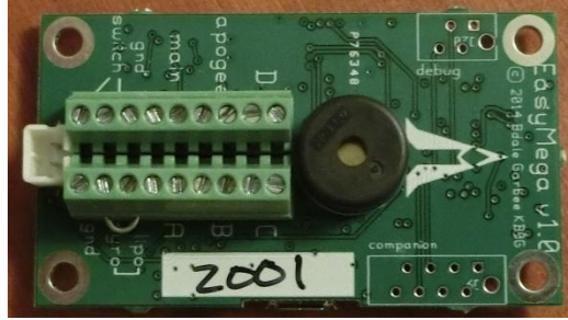
Figure 17: EasyMega Flight Computer
