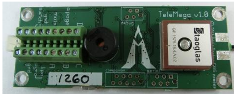
Figure 16: TeleMega Flight Computer
