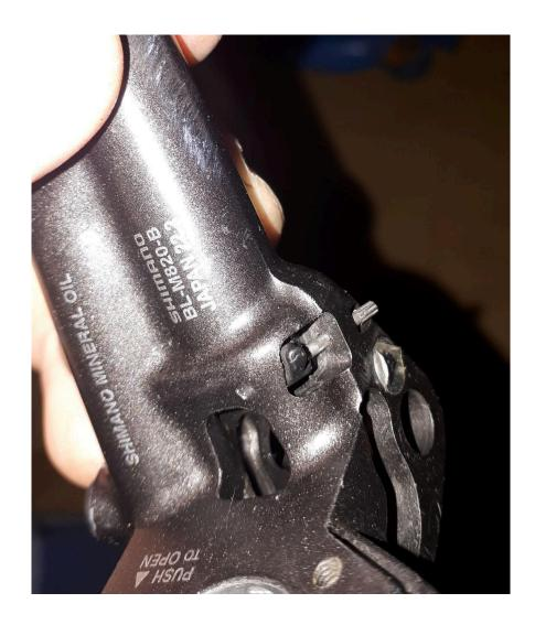
2.3. Loosen the free stroke adjustment until the adjuster pops out from below the screw. It may spring out and fly away so it helps to put a tool through as you undo the screw, or hold a finger on top of the piston opening.
