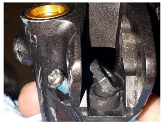
2.4. Now the piston may pop out on its own. Otherwise, use air pressure from a compressor (it may get dirty!) or a blunt tool pushed through the opening for brake hose to push the piston out, paying attention not to scratch the inside of the master cylinder with the tool.
