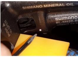
2.2. Once a part of the pin is sticking out, use pliers (vice grips may help) to pull the pin out
