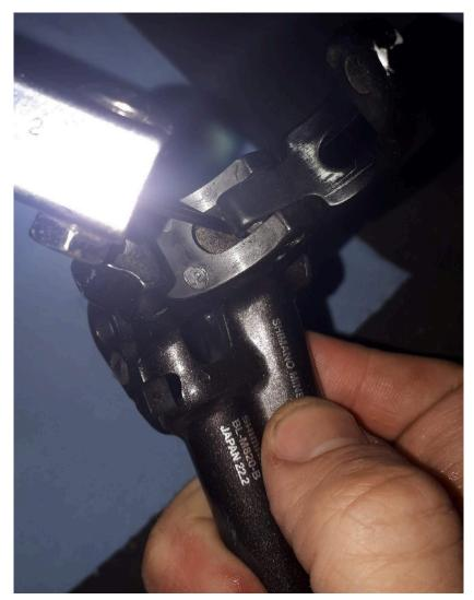
3.2. Use a 4mm bolt threaded into the end cap to remove the reservoir cap and bladder
