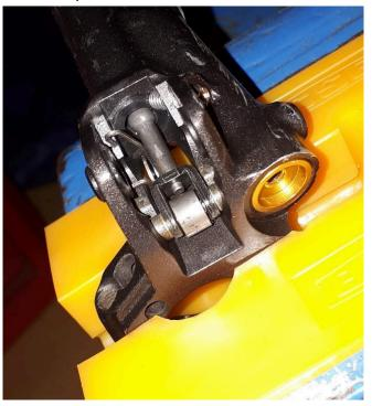
1.6. Push out both bushings using an allen key or a round tool of the right diameter and then pull up/wiggle on the ServoWave mechanism to pop it out. Notice the taller bushing goes on the bottom of the lever.
