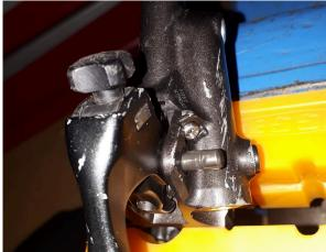
1.3. Push out the lever pivot pin while holding the lever, which will be free once the in is removed
