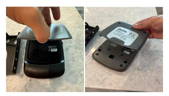
Step 3. Attach Skale 2 to the supplied Caddy piece. Placing the 2 front tabs on the slot first then pressing down to lock into place. (See Picture)
