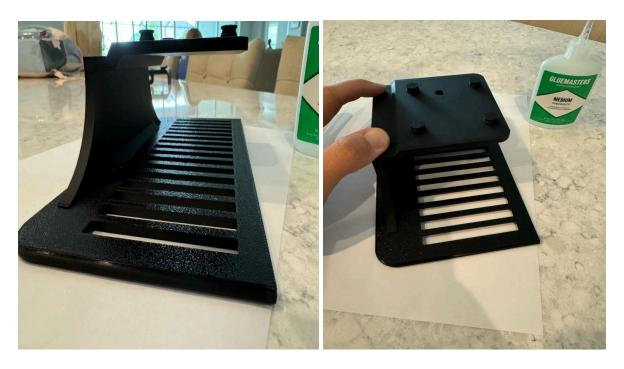
Step 7. Let glue dry for approx. 30-60 minutes to bond properly before finishing the assembly.
