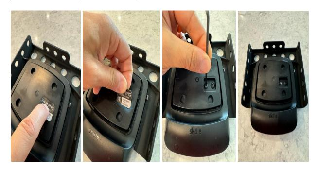
Step 10. Install the Adapter Base onto the Skale 2 and re-use bolt that was removed, be sure to only snug the bolt \*DO NOT OVERTIGHTEN\* (see below)
