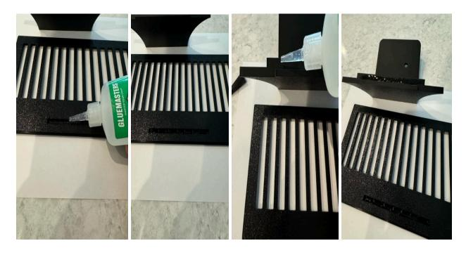
Step 6. Assemble the Adapter Base to the Grate so pressure can be applied for glue to set (approx. 30-60 seconds as shown below)
