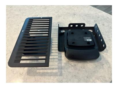
Step 9. Remove the "warning sticker" on Skale 2 and remove the Left bolt if facing the front of the scale. \*using a 3MM Allen Wrench \* Easiest way to get the sticker off is to push on the center. (as shown below)
