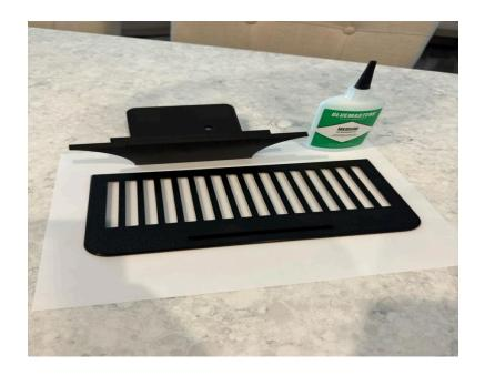
Step 5. Glue top Grate to Adapter Base, being careful not to use too much glue as it can get pushed out and not be aesthetically pleasing. (Apply only to the areas shown below.)
