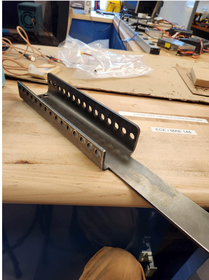
Fig 9: Fully Bent Lever Arm Laser Cut Out of Steel
