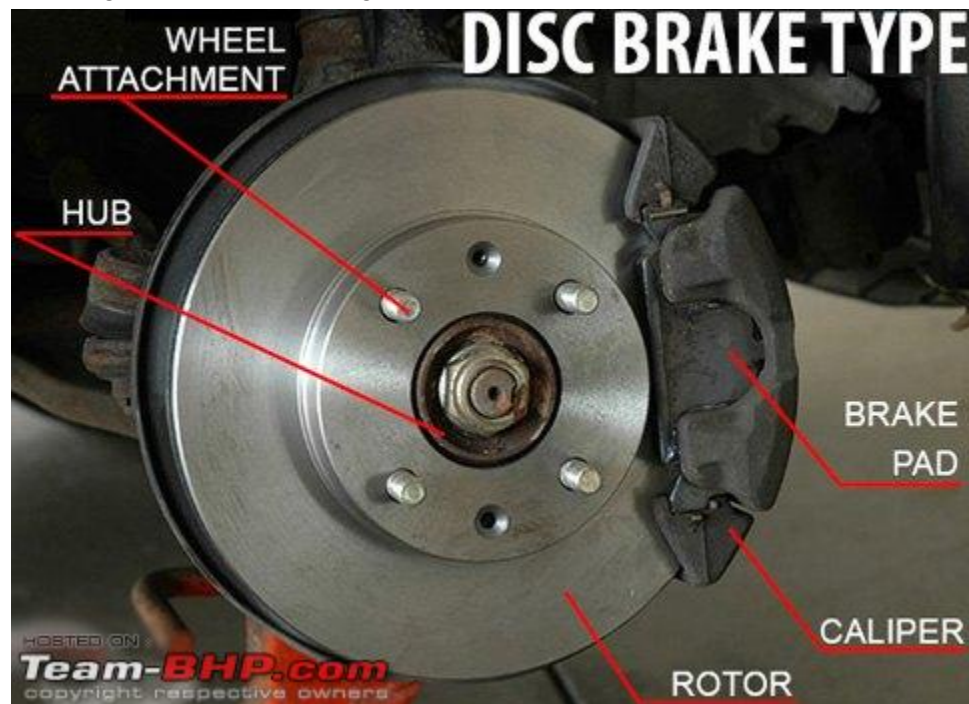
Figure B.3.1: How Calipers and Brake Pads are Attached (Appendix.A)
