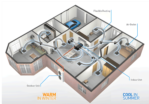
Central HVAC system
