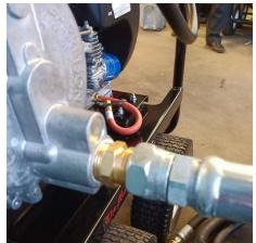
5. Attaching the Propane (LP) or Natural Gas (NG) hose to the fuel source. The other end of the hose must be connected to (1) the LP tank by inserting the reverse thread POL (located on the regulator end of the hose) into a propane tank using a wrench. Make sure the hose is secure. Or (2) the Natural Gas outlet. The NG hose comes equipped with a quick connect male located at the end of the
