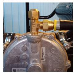
2. Connect and tighten the fuel hose fitting to the proper outlet.
