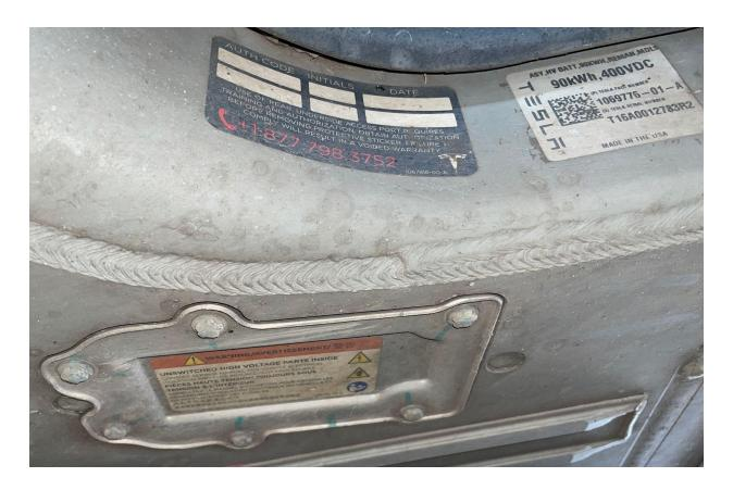
On V1.0 and V1.5 the cost will be much more expensive as the HV battery has to be dropped to access the fuse cover on the topside. This video shows why.
