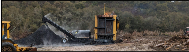
Carbonator (biochar kiln) processing eucalyptus at Elkhorn Slough Reserve; photo by Jamie Tuitele-Lewis
