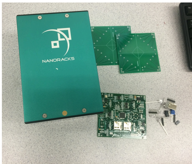
New Nanolab, NESI board, and sensors to replace the lost test module on CRS-7
