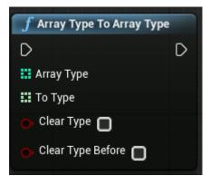
Transferring values to a different array of another type. Option to clear the array after operation and to clear before (the one that receives the values)
