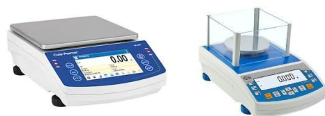
A top-loading balance (left) and an analytical balance (right). Note how many more zeroes the analytical balance has.
