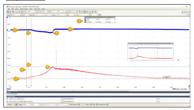
Channel A indicates the voltage of the O2 sensor Pump cell
