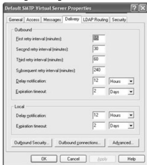
Figure: The Default SMTP Virtual Server Properties dialog box is where you configure SMTP settings.
