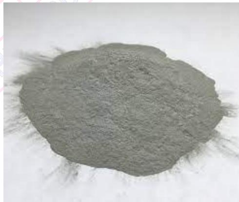
Tin powders are used to make bearings, friction brake pads, and chemical and industrial applications. When added to copper, tin powders largest use is in the production of PM oil-impregnated bronze bearings, but tin powder can also be found in plastics, solder pastes and other applications, such as diamond tools and abrasive wheels. It is used in the automotive, chemical, friction, metallurgical, pyrotechnic and defense industries.
