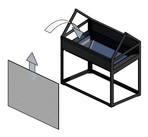
Adjust the glass, then secure the glass with the 2 fasteners provided by screwing them.
